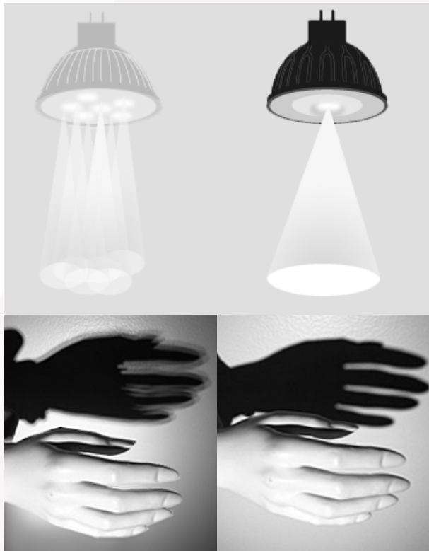
Figure 13. Soraa lamp's single light source (right) produces a beam free of the multiple shadows and colors typical of multi-source LEDs (left).
